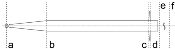
Fig. 8 Positions of constant x-planes for comparison of cross-section shapes of the cavity
