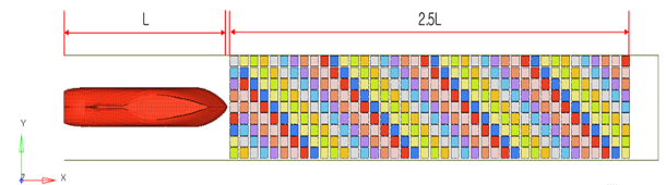
Fig. 6 Finite element model for towing simulation of a research icebreaker
