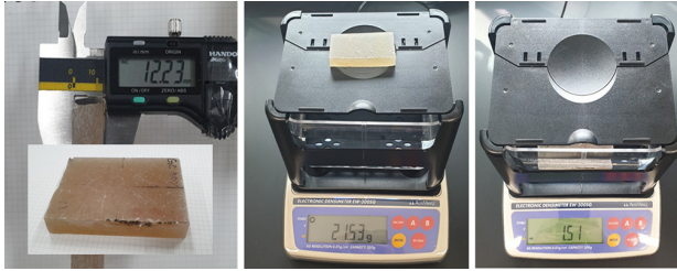
Fig. 4 Measurement of the relative densities from sample GFRP using a hydrometer
