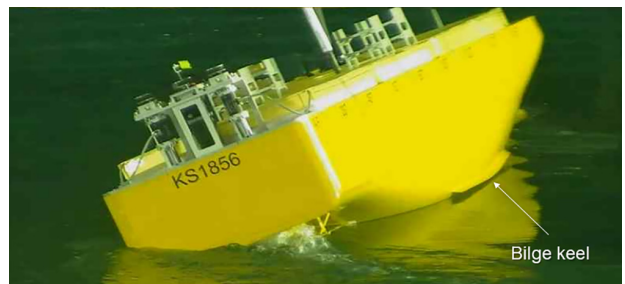
Fig. 13 Picture of bilge keel in -22 degrees heel angle
