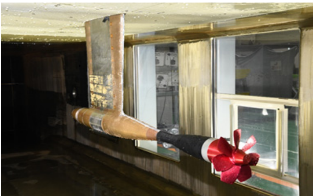
Fig. 13 Set-up for rotor-only open-water test (Rotor-only)
