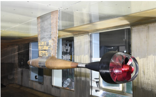
Fig. 12 Set-up for pump-jet open-water test
