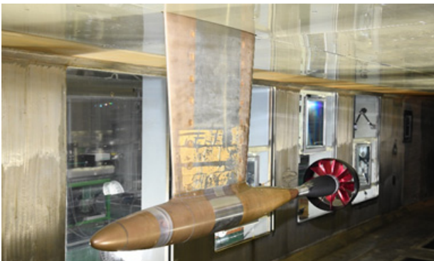
Fig. 5 The photograph of the H41 dynamometer
