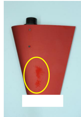
Fig. 2 Erosion damage (yellow circle) on the rudder surface
