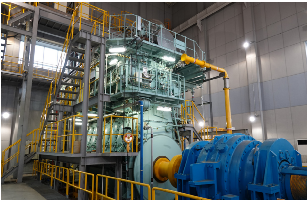
Fig. 1 2-Stroke low speed marine engine
