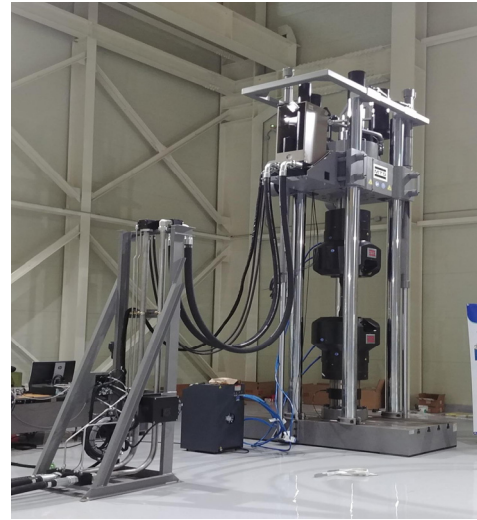
Fig. 5 MTS 2.5MN UTM(universal test machine)
