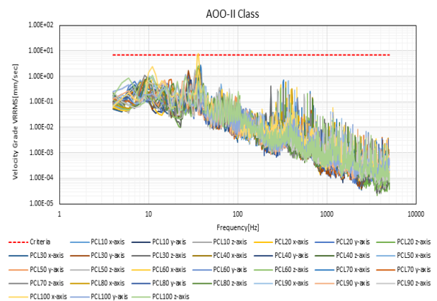
Fig. 12 Comparison of ABS, DNV criteria and vibration values of AOO-II Class
