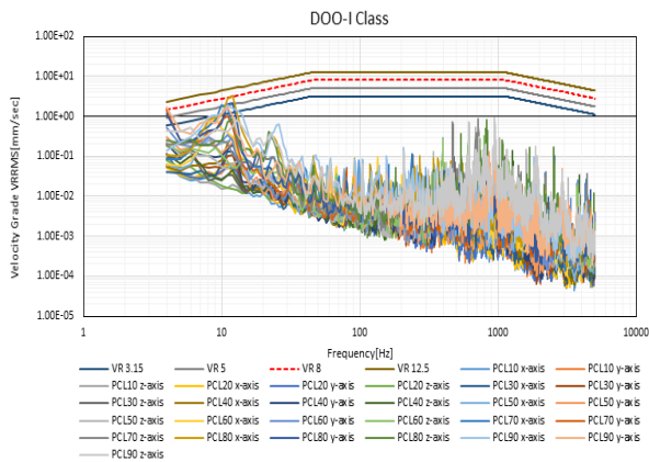
Fig. 25 Comparison of proposal criteria and vibration values of DOO-I Class (VR 8)
